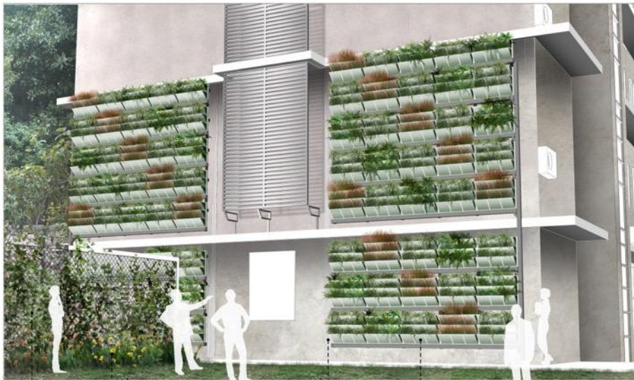
Green facade: Vertical flow wetland + Canna lily: Ornamental plants planted in the VF Feeding pipes: Pipes delivering greywater to the green Living wall: Green wall modules planted with ornamental plants treating
